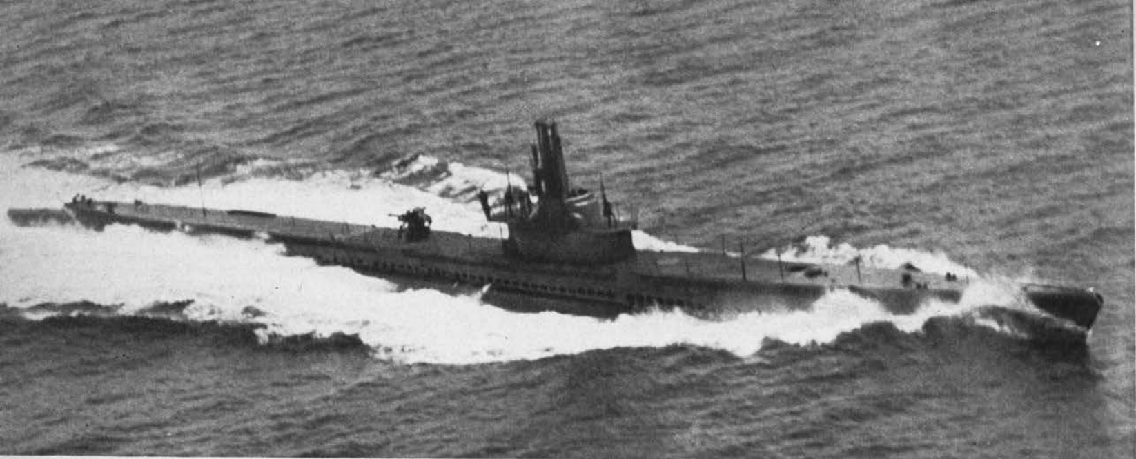
TALL HEAVY PERISCOPE SHEARS RISE LIKE STEEPLES FROM SQUAT MASS OF U. S. CONNING TOWER, DISTINGUISH OUR FLEET SUBS FROM ALL OTHERS
